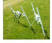
Frequent realignment of the instruments and zero drift correction ensure a constant high quality of data. Extremely sensitive, these instruments can detect variations in soil magnetism to 0.1nT, affording diverse application throughout a variety of archaeological, soil morphological and geological conditions.
